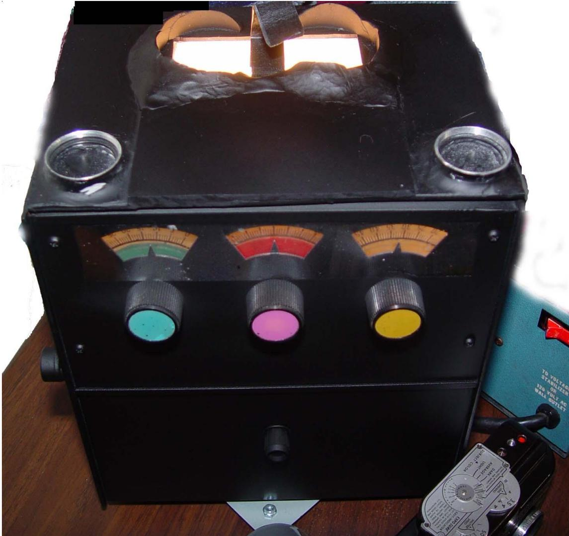
A few final touches were needed. I added a pair of Series V threaded adapters on top of the unit to hold the special close up lenses so I wouldn't lose them when the unit was in storage. I also got an old meter and affixed it to a PVC tube so that I could measure the light levels transmitted by my originals. There is a surprising amount of fluctuation in density, even if the original slide "looks" normal. Measuring this allowed me to establish the exposure for each slide.
