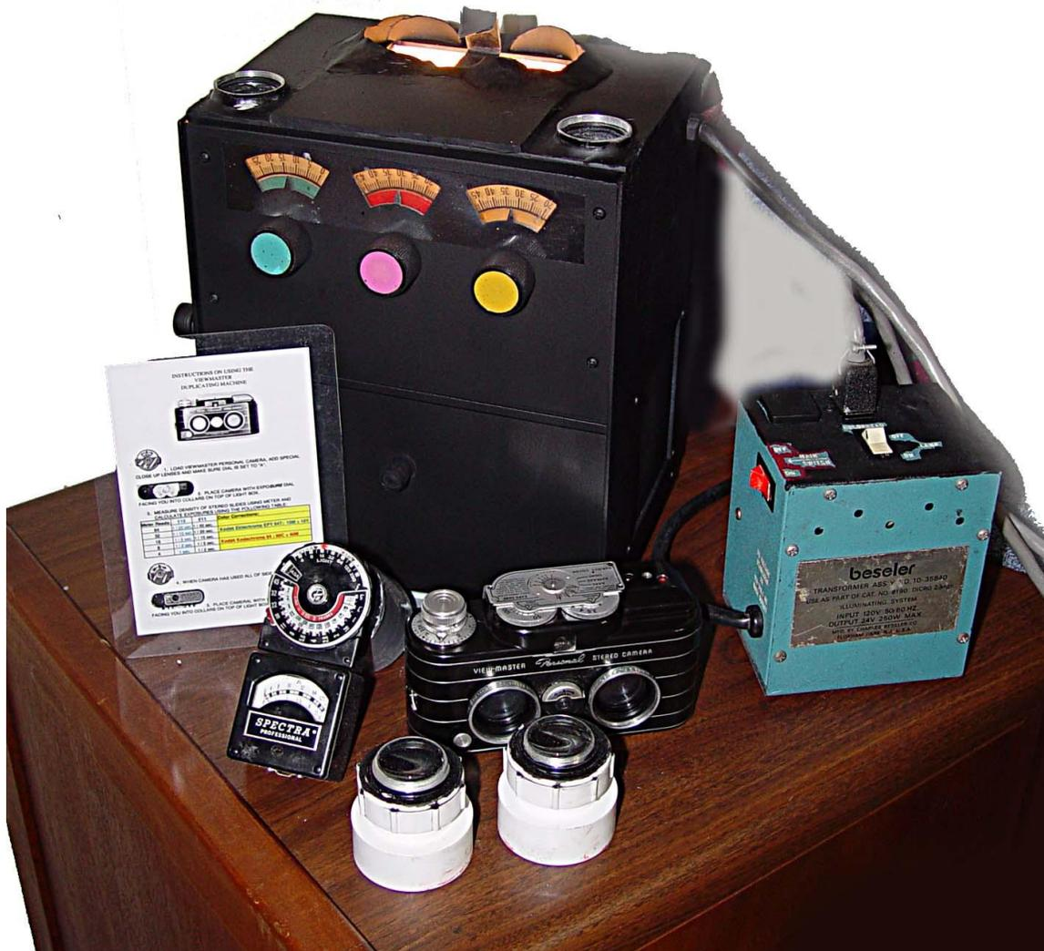
I still needed a set of close-up lenses that would give me high quality, or at least the highest quality, copies I could get. Using some optical formulas, trial and error, I finally found that a 48-50mm focal length lens would work. I decided on a 2-element achromat because I wanted the best color rendition. I obtained mine from Anchor Optics, a subsidiary of Edmund Scientific in NJ.
